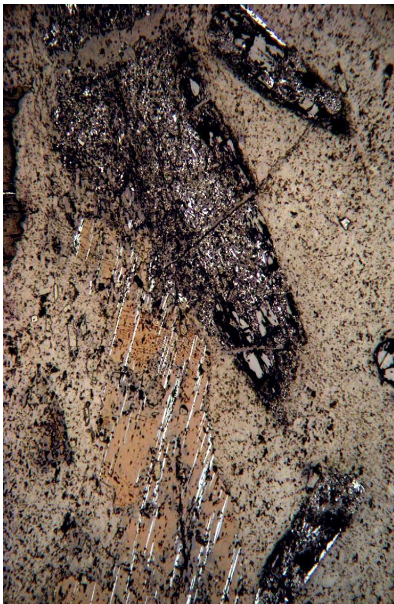
GD 69A Photo IMG-1658: Reflected light; same field as IMG-1657. Shows ferruginisation, in the form of diffuse impregnations of minutely fine-grained hematite (whitish grey), in the altered prismatic grains. Thin cleavage-related lamellae of Fe or Fe-Ti oxides are developed in the biotite.
